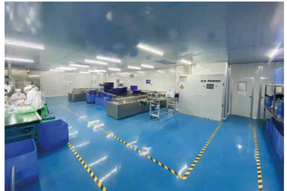
Self-built PC vacuum aluminum plating workshop, One spraying production line, two vacuum plating machine, 1000 level purification workshop
